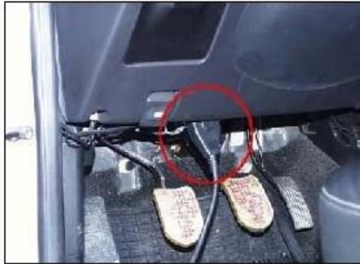
-Location of OBD-II diagnostic connector-
